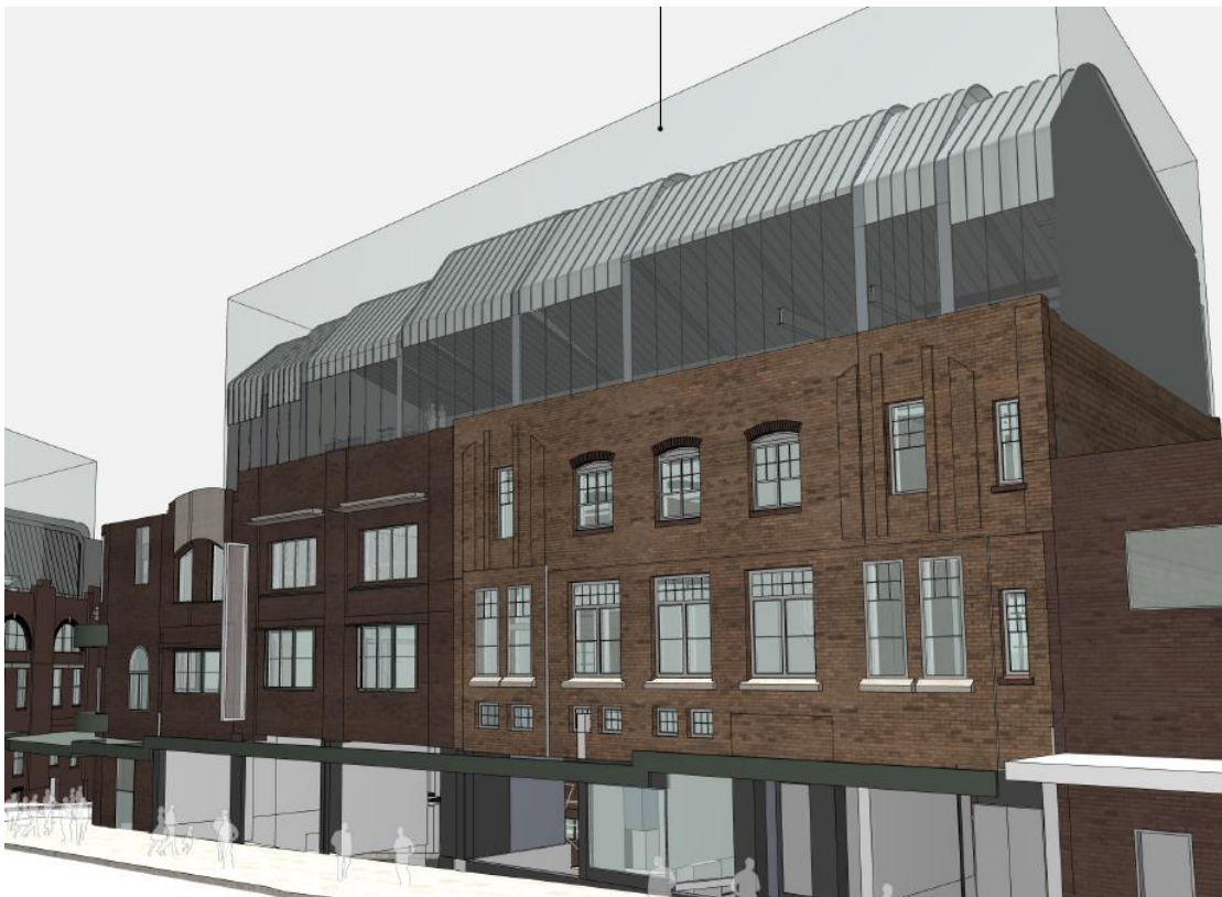
Figure 20: The alternative roof form shown with the draft DCP maximum envelope overlay (grey wireframe)
