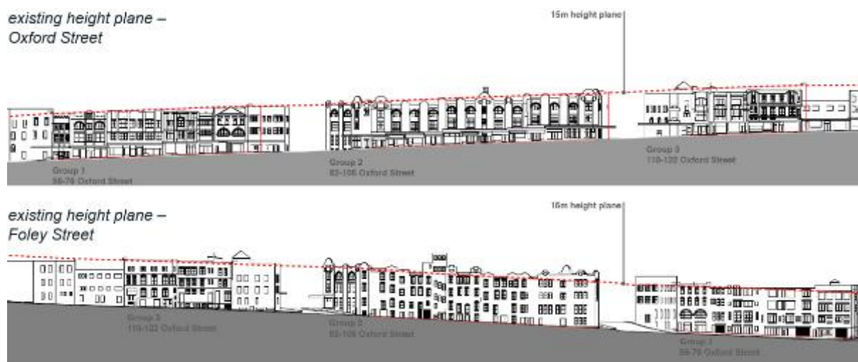
Figure 10: Existing height planes of Groups 1-3, shown in red, viewed from Oxford Street and Foley Street
