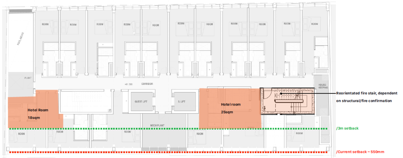
Figure 16: Setback analysis - alternative Level 3 plan. The red line indicates the proposed setback and the green line indicates the 3 metre setback.
