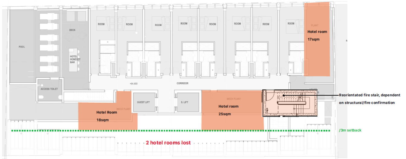
Figure 17: Setback analysis - alternative Level 4 plan. The green line indicates the 3 metre setback.
