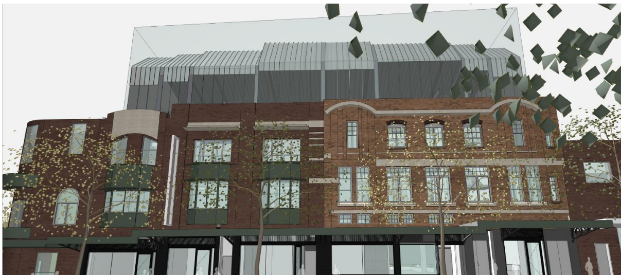
Figure 22: The alternative roof form shown with the draft DCP maximum envelope overlay (grey wireframe)
